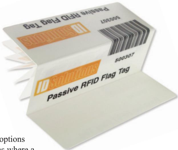
A great alternative to metal mount options or applications where a standoff will not work. Metalcraft's RFID Folded Tab Tag consists of an adhesive label that protects the encapsulated inlay and a non-adhesive, folding tab that offsets the inlay. The label has three sections: a middle section housing the RFID inlay; one end adheres to and provides extra protection for the inlay, while the other end adheres to the asset being tracked.
